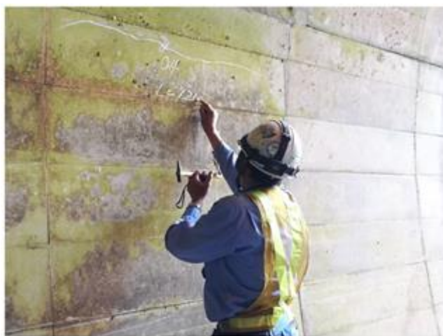
Fig. 1: A human inspector conducts the hammering test in a tunnel.
