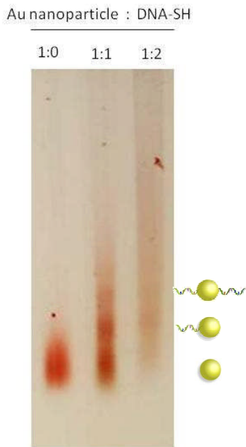
Fig. 3. three wt% agarose gel electrophoresis of DNA-SH bound to Au nanoparticle (molar ratio AuNPs : DNA-SH = 1 : 0 – 2)
