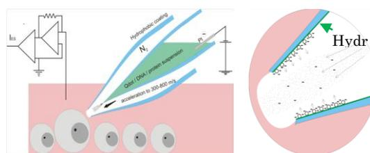
Figure 1: (Left) Concentric nanoelectrospray design and measurement setup. The inner pipette contains the solute to be ionized (Qdot/DNA/protein suspension). (Right) Coulombic repulsion causes droplet fragmentation into smaller droplets, accelerated in the electrical field. Initial immobilization of charged droplets on the hydrophobic surface of the outer pipette creates repulsion and focusing of the ion plume toward the exit.
