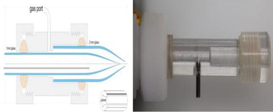
Figure 2: Design and micro-fabrication of a holder for concentric glass capillaries. Note the presence of a gas port allowing the creation of an internal pressure in the gap between the two capillaries. High voltage is applied to the solution through a platinum wire inserted to the back of the inner pipette. Materials (Teflon, polycarbonate) were selected for their high quality as insulator.
