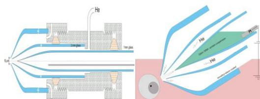
Figure 6: Proposed alternative design for sheath flow-assisted electrospray. Three concentric tapered capillaries allow a continuous flow of dry gas, drying droplets deposited on pipette surfaces and providing additional velocity to the electrosprayed polymers. Gas escape and gas pressure are calibrated to regulate sheath flow and keep a stable interface between the saline and the aperture of the outer pipette.
