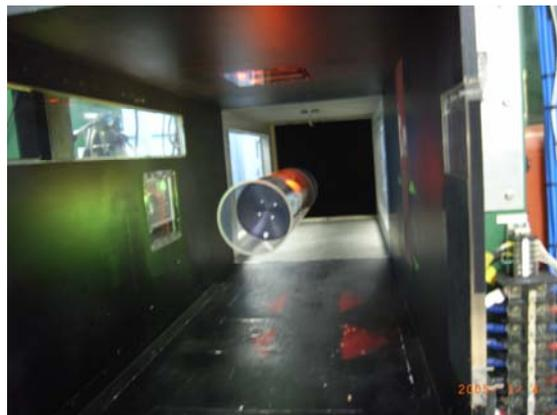
A cylindrical model magnetically suspended in the JAXA 60 cm MSBS wind tunnel.
