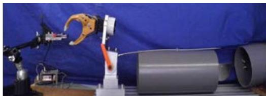
Fig.1 Experimental setup for the myoelectric control
