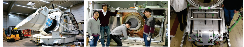
Figure 2. Instrumental achievements prior to this research: telescope mount, cryogenic optics tube, and calibration system.
