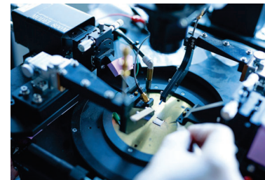
Figure 2 A system for experimental investigation of spin and orbital currents
