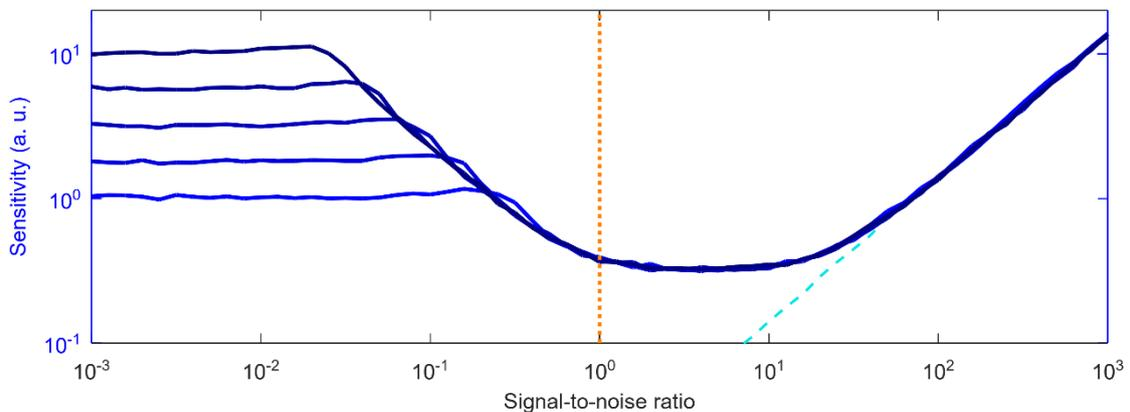
**Figure 3:** Sensitivity. At the centre, when the SNR is about 1, the sensitivity is the same as for conventional methods. For higher SNR, the randomness of the signal dictates the sensitivity, while for lower SNR, the randomness of the noise is the limiting factor. Please note that the measured signal is as in Figure 2, hence conventional methods cannot sense the signal at all.
