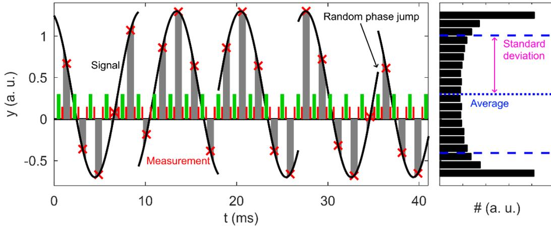
**Figure 2:** Standard-deviation quantum sensing method. (Left) When the signal has random phase jumps, conventional methods that accumulate data over multiple periods will find an average of zero. (Right) However, by measuring the standard deviation instead, the amplitude of the signal can be found. For example, for a sinusoidal signal, the relation between the amplitude  $A$  and the standard deviation of the signal  $\sigma$  is  $A = \sqrt{2}\sigma$ .
