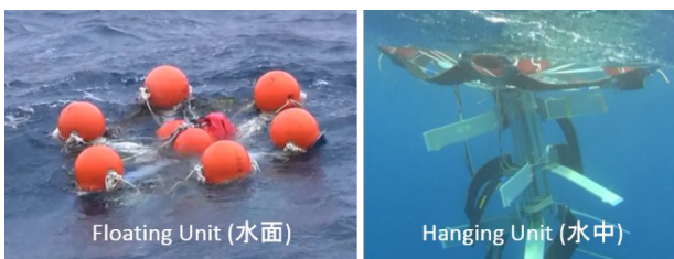
Fig.7 Field test in Okinawa, 2013. The diameter of the floater is about 40cm (Left: Floating unit, Right: Hanging unit)
