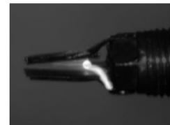
(a) Streamer discharge (Non-thermal plasma) w/ mica plate
