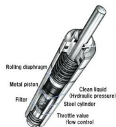
Fig4 Inner structure of dashpot
