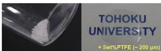
**Fig. 1** Typical photographs of the quasi-solid-state composite powder, 75 vol%(1MLi-TFSA – EMI-TFSA) – fumed silica, and the self-standing sheet, 95 wt%({75 vol%(1MLi-TFSA – EMI-TFSA) – fumed silica} – PTFE).
