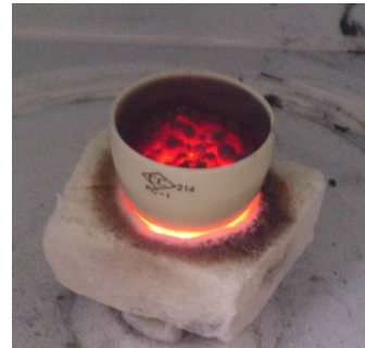
Fig. 8 Appearance of mixture after 4 min microwave heating (funnel glass=1 g, carbon 1=0.1 g)
