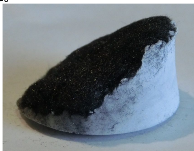
Fig. 7 Mixture of funnel glass and carbon 1 after induction heating
