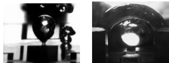
(A) 0.01MPa at ONB (Cu Film) (B) 0.01MPa at CHF (Cu Film) (C) 0.01MPa at ONB (Si wafer) (D) 0.01MPa at CHF (Si wafer) Fig.3 Behaviors of Bubble
