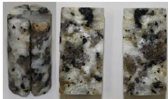
Photo 1. Granit specimen which includes tensile single fracture
