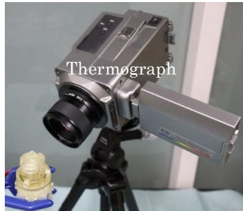
Fig. 6 Response measurement by thermography
