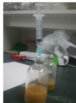
Measure gas production
