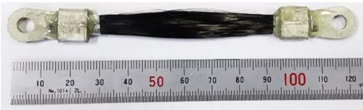
Fig.6 Photograph of carbon fiber sample with chucking terminal.
