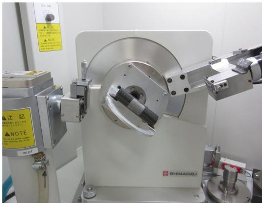
Fig.10 Photograph of x-ray stress measurement. CFRP pipe sample sets on the  $\Omega$ -diffractometer system.
