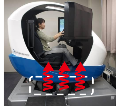
併進方向:3自由度(x,y,z) 回転方向:3自由度(roll, pitch, yaw)
