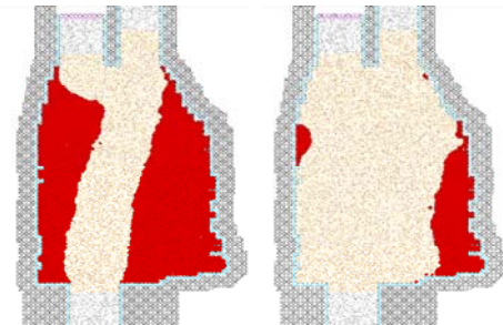
Fig.4 Simulation result of thrombus formation without (left) and with (right) dosage
