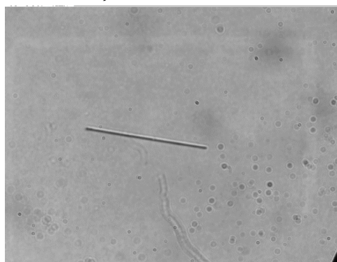
Fig. 4 Optical image of silicone nanowire.
