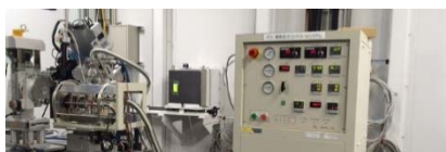
Figure 3: Sterling refrigerator and gas dosing apparatus.
