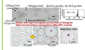
Figure 3. High through-put production of DNA-functionalized nanoparticle (DNA-NP) crystals using microfluidic channels
