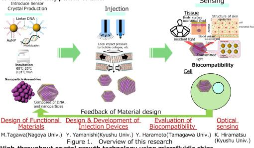
• High-throughput crystal growth technology using microfluidic chips We have the technology to grow DNA-functionalized nanoparticle (DNA-NP) crystals that function as sensors in a microfluidic chip as designed, and the technology to produce them at high throughput. Furthermore, we can also perform solution replacement to place the DNA-functionalized nanoparticle crystals in a biocompatible solution environment for use in vivo.
