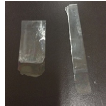
Fig. 4 Erosion of a cover glass (left) and a slide glass (right) (O mark)
