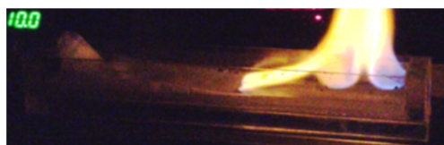
Fig.7(a) Extinguished cover the electrolyte surface (Exp.No.5)
