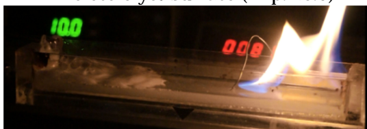
Fig.7(b) Extinguished before the foam hits (Exp.No.6)
