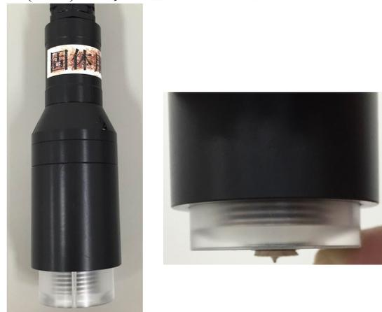
Figure 3 Thermal probe with instantaneous point contact (thermophysical handy tester).
