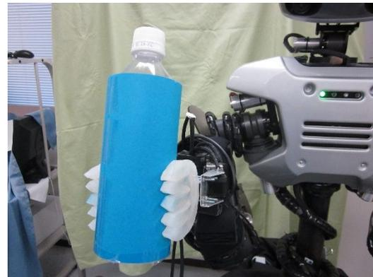
Figure 2 Robot hands developed by Yamano's group using the SMG of Furukawa's group.
