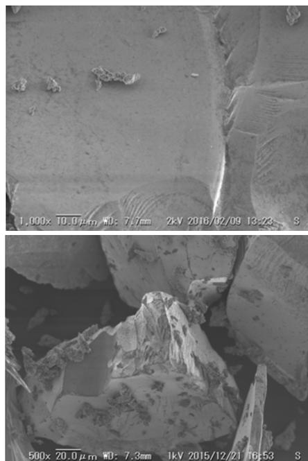
Fig.5 SEM images of surface of milled SiC particles. Applied Cu particle was (upper) not milled and (lower) milled, respectively.
