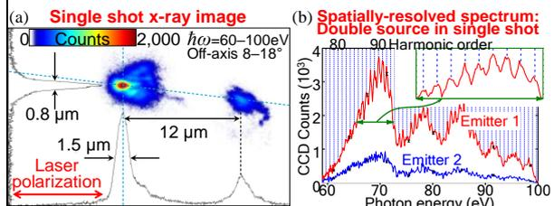
Fig. 5. Single-shot image (a) and spatially-resolved spectrum (b) of the BISER x-ray source (Experiment) [5].
