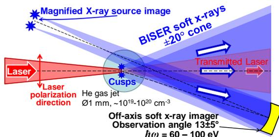
Fig. 4. Experiment schematic. Laser pulse irradiates helium gas jet producing *density singularities* (*Cusps*) emitting bright coherent x-rays via the BISER mechanism with a wide angular distribution. An x-ray imaging mirror intercepts off-axis radiation ( $8^\circ$  to  $18^\circ$  off-axis) and images with magnification the source onto a LiF crystal detector [5].
