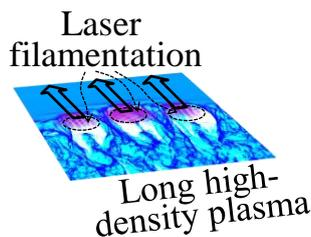
Fig. 2. Laser filamentation in a usual high-density gas jet. The blue scale shows the electron density.
