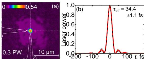
Fig. 7. J-KAREN-P laser spot (a) and pulse (b) [6]; the dashed line in (b) is the bandwidth-limited pulse.
