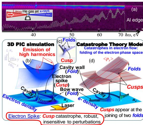
Fig. 1. (a) Typical single-shot harmonic spectrum (experiment, J-KAREN laser); (inset) experimental setup. (b) 3D PIC Simulation: Relativistic singularities (density spikes) and harmonics emission (red arcs,  $\omega \geq 4\omega_0$ ); for higher harmonic orders, the arc length reduces resulting in *two point-like sources*. Inset (c): Discrete particle model result. (d): *Catastrophe Theory Model*: folds of the phase space lead to *catastrophes* (density singularities).
