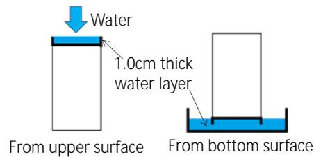
Fig. 2 Water absorption experiment
