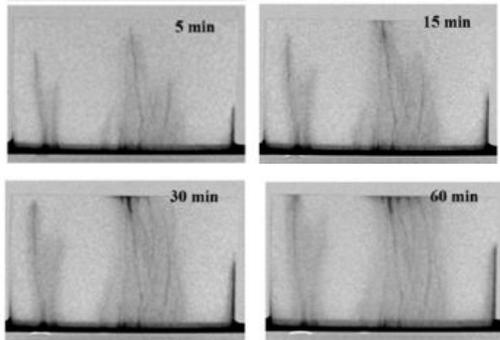
Fig. 8 Observation of water propagation in cracked ECC (Experiment from Zhang et. al 2010, *Observation and quantification of water penetration into strain hardening cement-based composites (SHCC) with multiple cracks by means of neutron radiography*)
