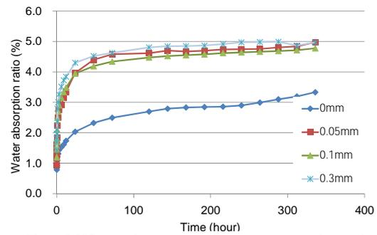
Fig. 5 Water absorption from upper side with various crack widths
