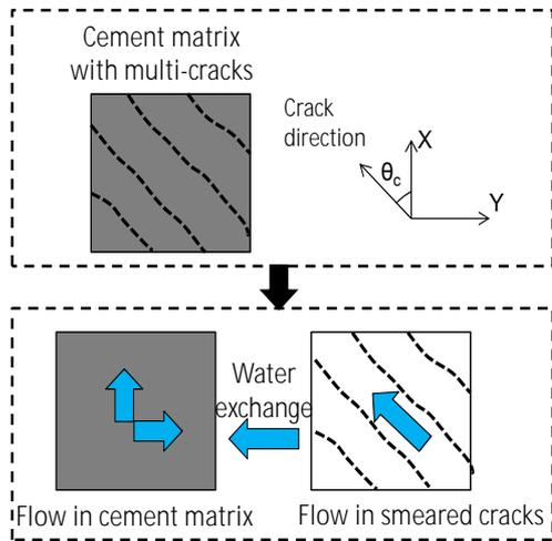
Fig. 3 Scheme of the two-phase model
