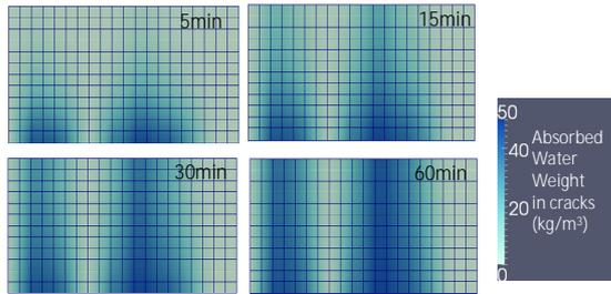
Fig. 7 Water contours in cracks using area-localized distribution analysis
