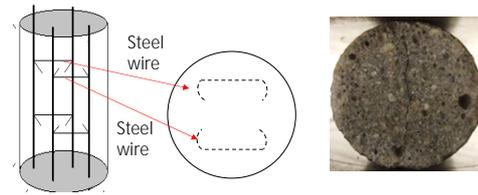
Fig. 1 Crack induction method
