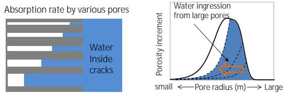
(a) Water ingress into pores with various radii (b) Water ingress into the entire pore-structure
