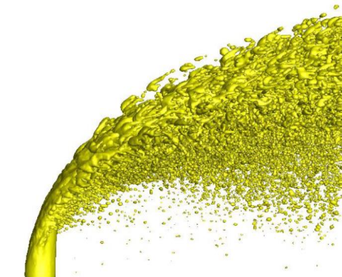
Fig.14 The primary breakup of liquid jet in a transverse wind field.
