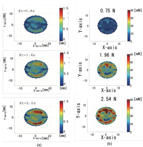
Fig. 3: Dynamic change of distribution of lateral force and traction over time under operation of the multiple haptic pins. (a) All pins are given with pre-determined lateral displacement that conforms to LDP: inner node with 1 mm, middle nodes
