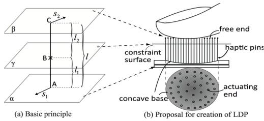
Fig.1: Illustration of principle for generation of localized displacements on human fingertip
