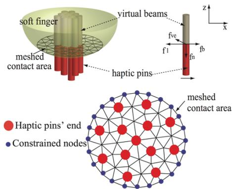
Fig. 2: Dynamic model of haptic pins making contact with virtual beams of the fingertip.
