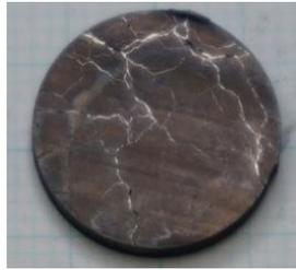
Fig.1: Photograph of the MgB<sub>2</sub> bulk #1.
