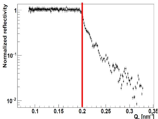
Fig. 2. The reflectivity plot for the NiP (10%) sample.
