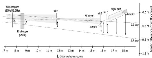
Fig.1. Schematic view of the SOFIA reflectometer. Taken from [5]
