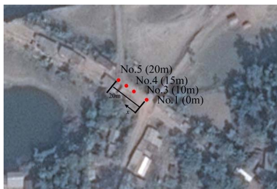
図 1(a) Morigaon (Assam 州) 破堤河川堤防 実施試験：DCP, MASW
