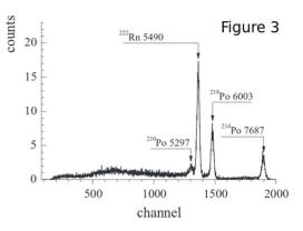
(Figure 3) will be used to identify 5490keV α-particles from decay of <sup>222</sup>Rn in the air.
