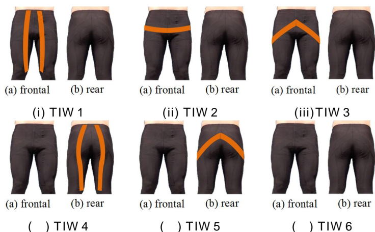
Fig.3 Prototypes varying the layer pattern of tap-shaped knitted fabric
