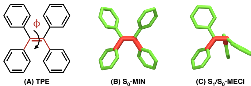
Figure 1. (A) Chemical structure of TPE, (B) local minimum structure optimized at the electronic ground ( S_0 ) state ( S_0 -MIN), and (C) structure at the minimum energy conical intersection between the S_0 and first excited ( S_1 ) states ( S_1/S_0 -MECI).
