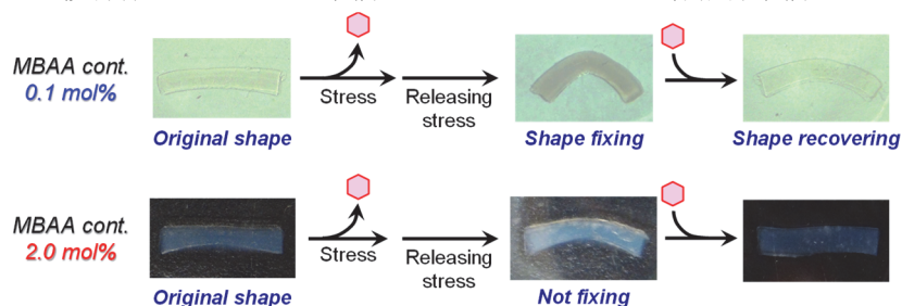
Fig. 5. Series of photographs showing the macroscopic shape-memory effect of PGEMA-PBA semi-IPN hydrogels with a MBAA content of 0.1 and 2.0 mol%.
