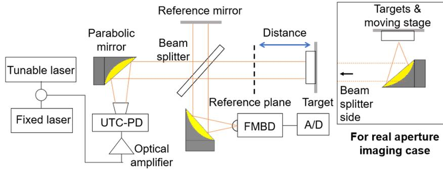
**Fig. 2.** Experimental setup of the THz FMCW system.
