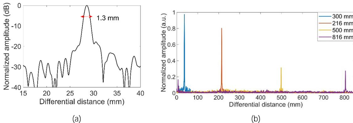
**Fig. 3** Signal characteristics of the proposed system: (a) reflected time-domain signal from a mirror at a 28-mm distance; (b) sensing results with a metal reflector placed at different distances.
