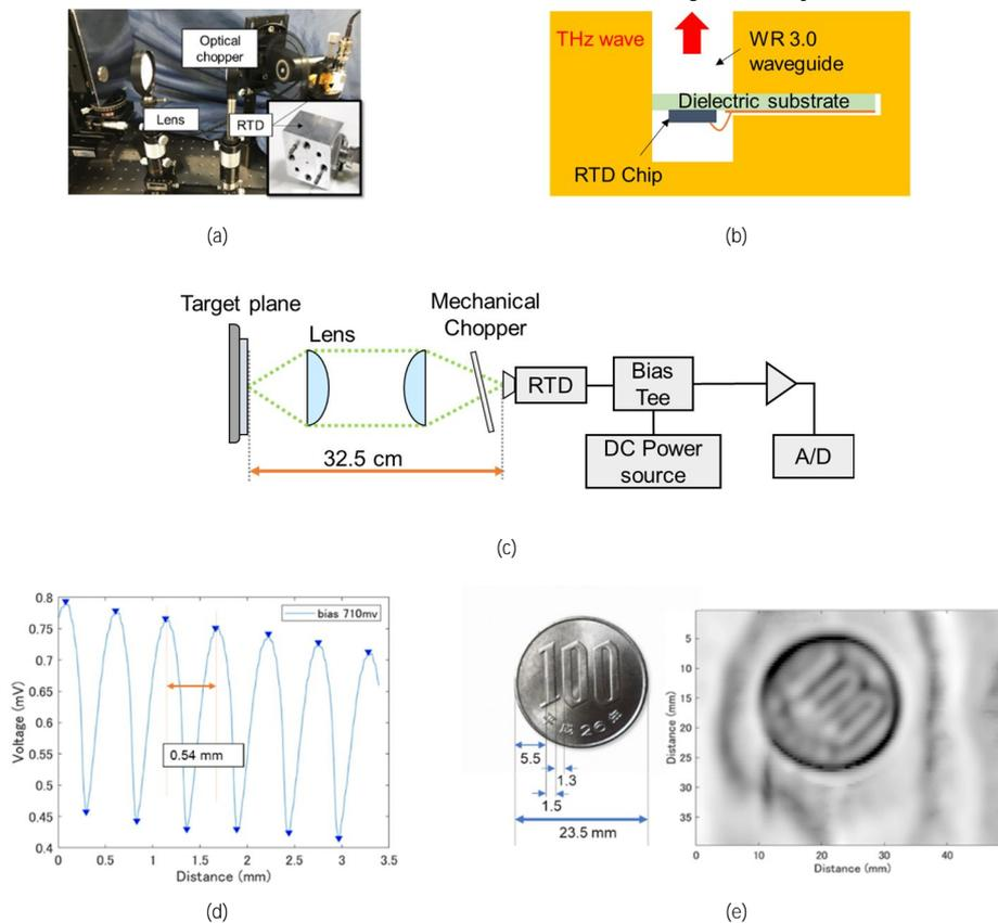
**Fig. 1.** Demonstration of a single RTD transceiver for imaging application; (a) Experiment setup; (b) concept of the waveguide integrated RTD (b) block diagram of experiment setup; (c) coherence signal obtained by moving the reflector; (d) imaging result of a 100-yen coin, ~1 mm spatial resolution can be obtained.
