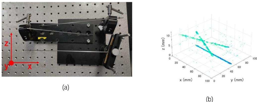
**Fig. 4** SAR imaging result of the 3D distributed rods: (a) imaging model; (b) top-view of the 3D-imaging result.
