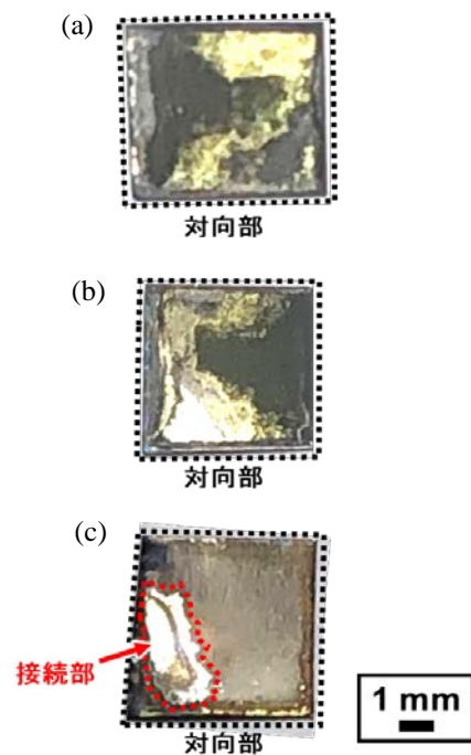
Fig.10 Photographs of film surface after peeled-off of the jointed samples at (a) 50 Pa, (b) 500 Pa, (c) 5000 Pa.
