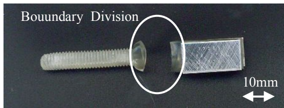
Fig. 3 Tensile fracture specimen in pull-out test.
