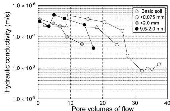
Figure 7 Variations in hydraulic conductivity with continuous permeation. The figures in the legend denote the particle size fraction of the stabilising agent used for the amendment.
