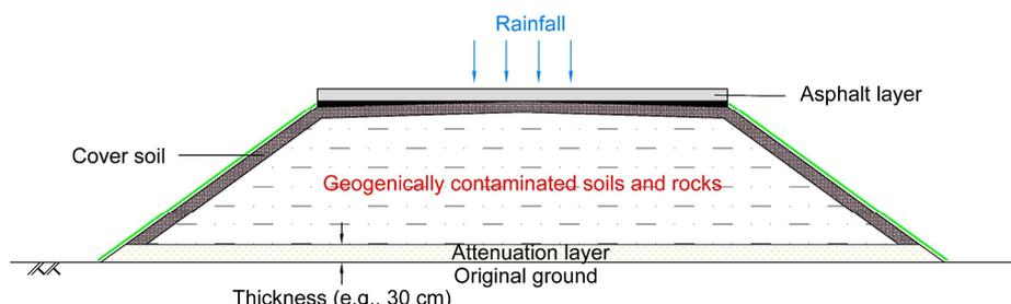
**Figure 1** Schematic diagram of an embankment installed with an attenuation layer underlying geogenically contaminated soils and rocks.
