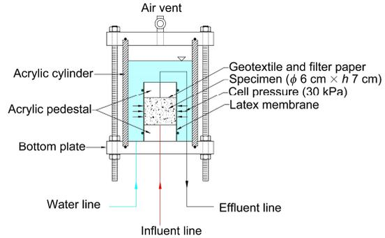
Figure 3 Schematic diagram of the flexible-wall permeameter.
