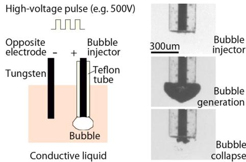
Fig. 2 The bubble injector for the generation of microbubbles
