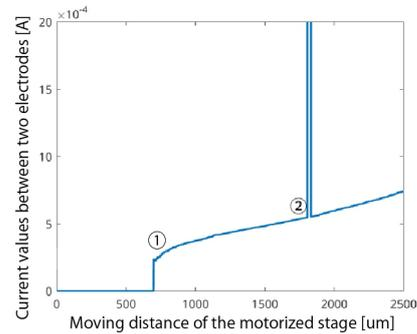
Fig. 3 The tip of the bubble injector is sequentially moved from the air to the surface of the egg white ① and then to the surface of the (CAM) ②
