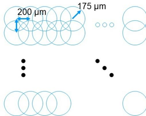
Fig. 5 Formation of a large area with cell removal on CAM. Each time the stepper motor moves 200 μm to the right or downward, bubbles are generated to treat the CAM, ultimately creating a large area of cell removal on the CAM
