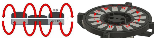
Fig. 2 Difference in appearance of magnetic lines of force between (a)normal magnet and (b)proposed device
