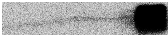
Figure 2 3 H β-ray image of 3 H @ TiO 2 -modified ITO electrode on imaging plate (IP). An FLA-9000 imaging scanner with 50 µm resolution was used.
