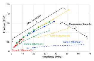
Fig. 3 Measured and corrected curves of iron losses with core A to D. [3]
