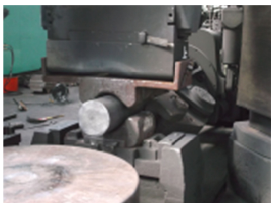
Fig. 7 Hot forging of large size high tin bronze ingot for mass production.
