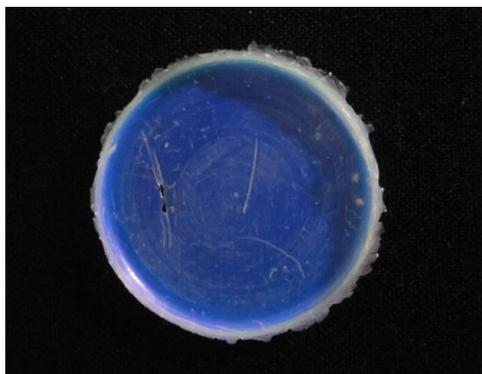
Fig 4. Photo of a bulk cast-film of high molecular weight block copolymer.
