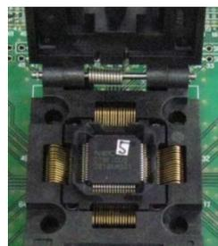
Fig. 3 Digital processor inside digital processor board
