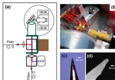
**Fig. 1.** (a) STM-TERS system inside an environmental enclosure. The illumination/detection optical paths are both fiber coupled. (b) Tip and sample junction illuminated by 633 nm laser through the objective lens. (c) STM tip under optical microscope. (d) SEM image of the tip with diameter  $\sim 40$  nm.
