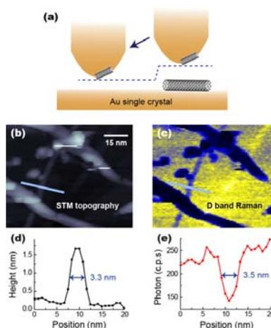
**Fig. 6.** (Left) STM topography of SWNT and its line cut across a single tube. (Right) Near field Raman imaging shows reversed contrast from usual TERS. The Raman imaging shows high spatial resolution as the STM topography.
