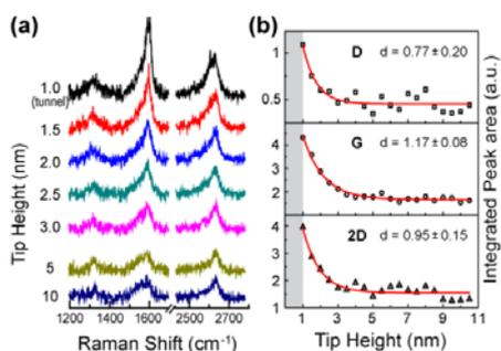
**Fig 5.** (a) Series of spectra taken at location 1 of CNT-1 of Fig. 4a while retracting the tip away from substrate at 0.5 nm/step. The integration time of each spectrum is 1 second. (b) Evolution of integrated peak area fitted with single exponential decay versus tip height of three Raman bands.
