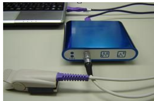
Fig. 1 Finger plethysmography equipment
